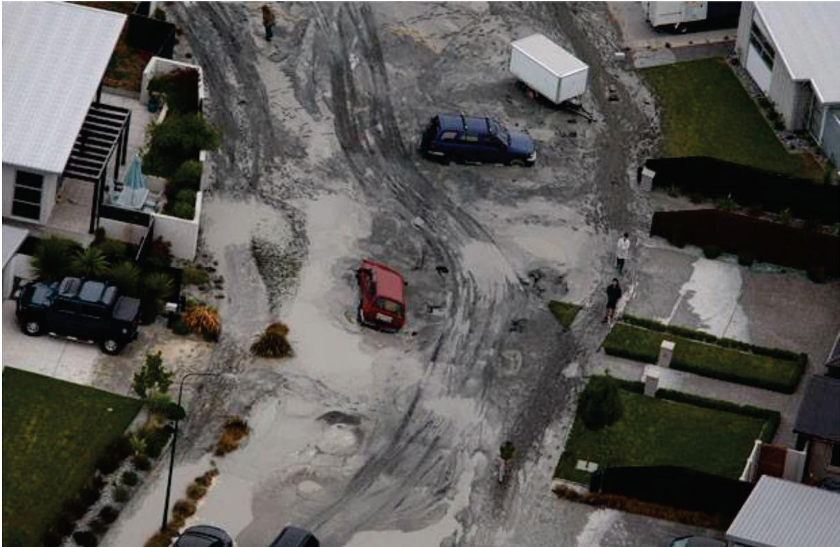
**Photograph 2.2** Liquefaction ejecta in a suburban Christchurch Street. In the suburb of Bexley, approx. 10 km from the epicentre after the magnitude 6.3 Christchurch earthquake of 22 February 2011 (Photo NZ Herald).
